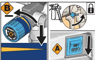
**6** Turn Pressure Control Knob to lowest setting and release trigger. Engage Trigger Lock. Move Prime/Spray Valve to PRIME and turn Power Switch OFF.
