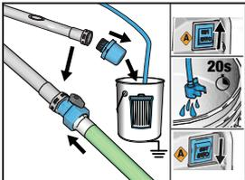
**4** Unscrew inlet screen and place in waste pail. Thread Power Flush Valve to Suction Tube. Open Power Flush Valve. Turn Power Switch ON and let water run through Drain Tube for 20 seconds. Turn Power Switch OFF.
