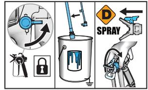
**7** When paint comes out of gun, release trigger. Engage Trigger Lock. Transfer Drain Tube to paint pail and attach to Suction Tube. Rotate Spray Tip back to SPRAY position and ensure Spray Tip Guard is tight.
