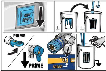
**1** Turn Power Switch OFF. Place Suction and Drain Tubes in waste pail. Move Prime/Spray Valve to PRIME. Turn Pressure Control Knob to START position. Trigger gun into a waste pail.
