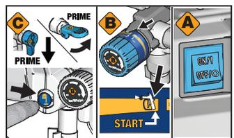
**3** Move the Prime/Spray Valve to the PRIME position. Press the PushPrime button\* twice to loosen inlet valve ball. Turn Pressure Control Knob to START position. Turn Power Switch ON.
