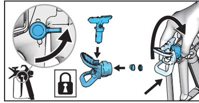
**2** Engage Trigger Lock. Assure Spray Tip is properly inserted into the Spray Tip Guard, and the Spray Tip Guard assembly is tightened securely to gun.
