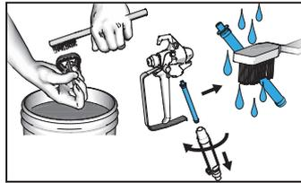
**7** Clean Spray Tip, Spray Tip Guard and inlet screen with brush. Remove gun filter and clean. Reassemble gun filter, Spray Tip and Spray Tip guard.
