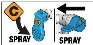
**6** Move Spray/Prime valve to SPRAY position for storage. Turn Power Switch OFF and unplug sprayer from outlet.
