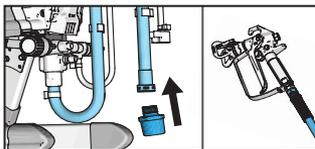
**5** Screw inlet screen back to Suction Tube. Ensure that spray gun and hose stay attached to sprayer.
