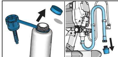
**1** Remove Pump Armor bottle cap and foil seal. If needed, unscrew inlet screen from Suction Tube.
