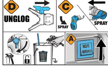
**6** Rotate Spray Tip to UNCLOG Position. Disengage Trigger Lock. Point gun into waste pail, pull and hold trigger. Move Prime/Spray Valve to SPRAY position and turn Power Switch ON.
