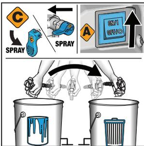
**5** To save paint in hose, disengage Trigger Lock and trigger gun into paint pail, move Prime/Spray Valve to SPRAY and turn Power Switch ON. When water comes out of gun, keep gun triggered and aim into waste pail. Continue to flush until water runs clear.
