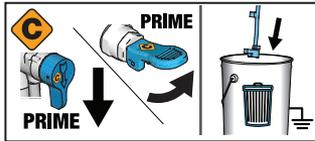
**2** Move Prime/Spray Valve to PRIME. Place Drain Tube in waste pail. Turn Pressure Control Knob to START position.
